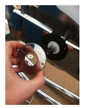
6)Remove the three screws and remove the stainless steel collar
