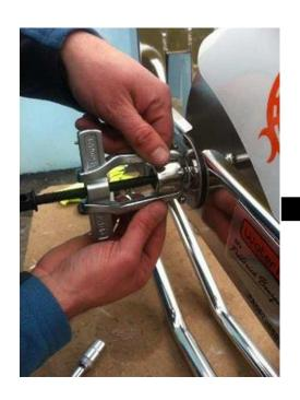
4)Disassemble the crank with a hub puller
