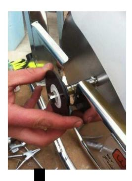
8)Remove the bearing and replace it
